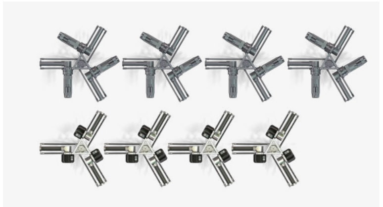
Smaller Footprint Traditional Servo-Gearhead Drivetrain vs LiveDrive Direct Drive Actuator
